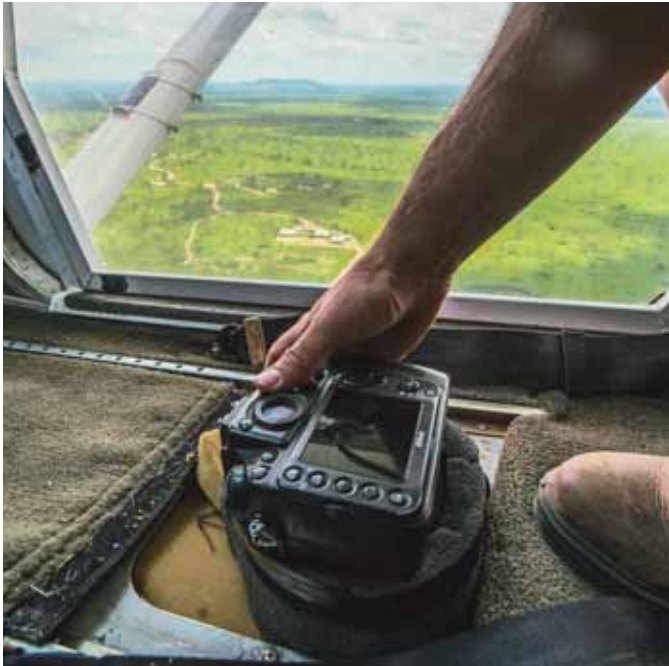
Using a camera fitted in the bottom of the aircraft, the herds of wildebeest are photographed and then counted using a computer.
