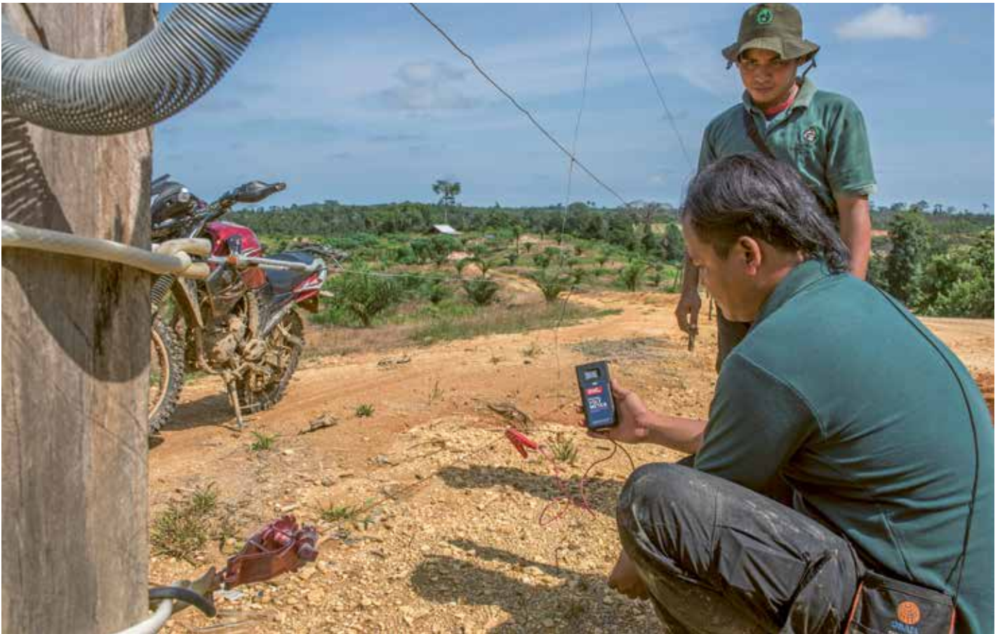
Albert Tetanus from the FZS team in Bukit Tiga Puluh testing the voltage on a solar-powered electric fence. This, in combination with other measures, is intended to keep the elephants away from fields and plantations in order to avoid conflicts.
